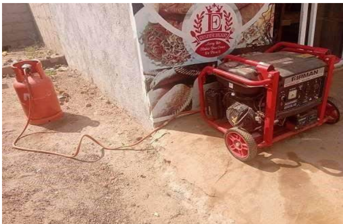
Plate 5. Converted Generator Used in Restaurant at Masaka, Karu LGA
